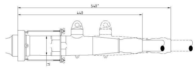
(\*) Minimum dimension required for disconnection
