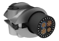
The cast iron claw cleat is the premium choice for fire performance cables. Suitable for all cable routes, the claw cleat can tolerate a two hour excursion of up to 1000°C.
