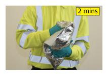
5. Tumble and knead the bag to mix the two liquids for up to two minutes.
