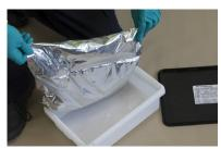
1. Open container and remove foil resin pack. Check bag for any signs of damage before proceeding.
